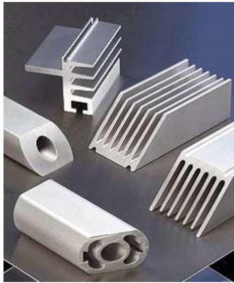
Figure 6. Examples of parts made by extrusion (each part is cut from a long length)
