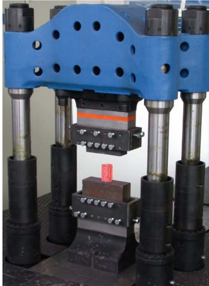
Figure 4. A simple forging press; note the red hot bar stock in place
