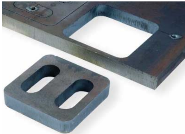
Figure 9. Thick steel sheet cutting using laser
