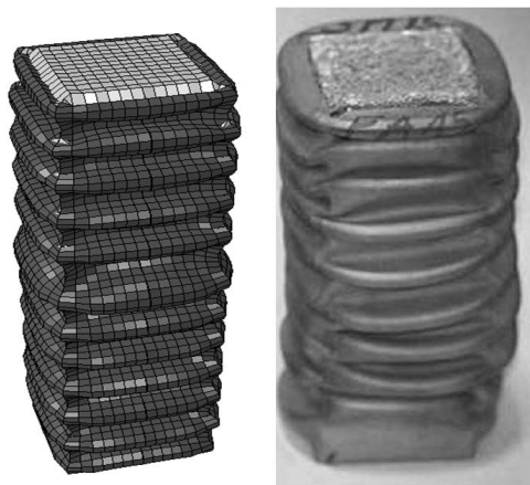
Fig5.. Comparison of experimental deformation [22] with numerical prediction.
