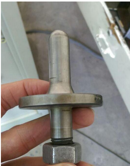
Fig2.Steel imp actor used in drop ball tests
