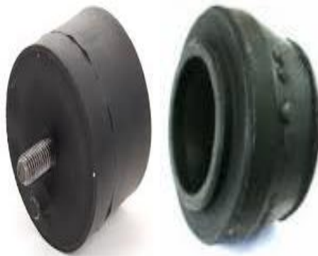
Fig23. Elastomeric Engine Mount
