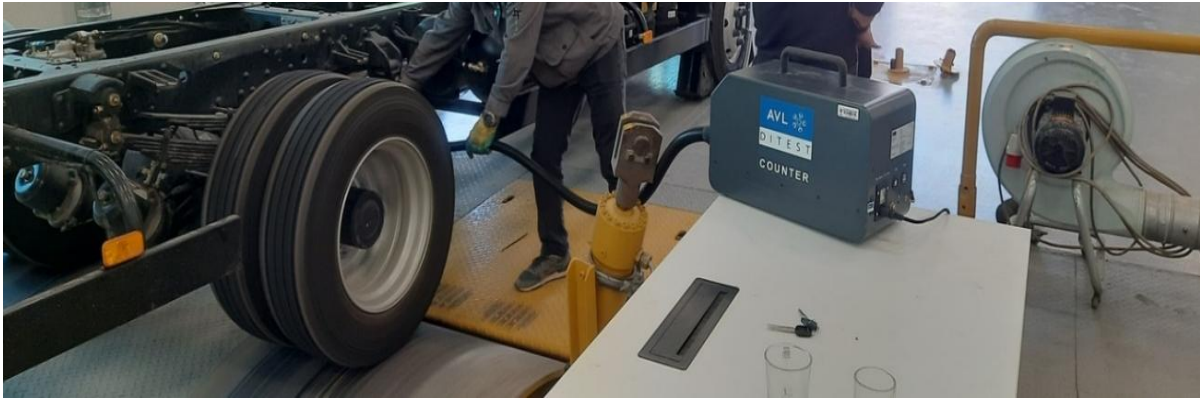
Figure 3: Device for measuring emitted particulate matter
