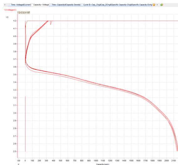
Figure 4: battery voltage profiles during charge–discharge cycles under vibration-exposed conditions.
