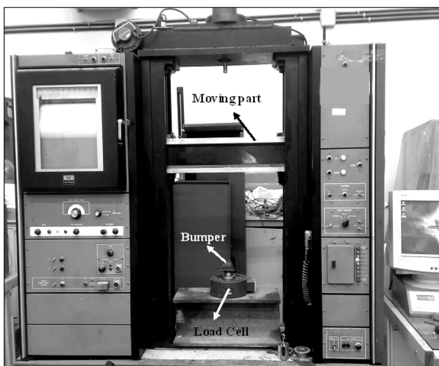
Fig. 10. Instron 1115 for the compression test of the bumper
