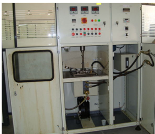
Fig16. Test setup of external gear pump
