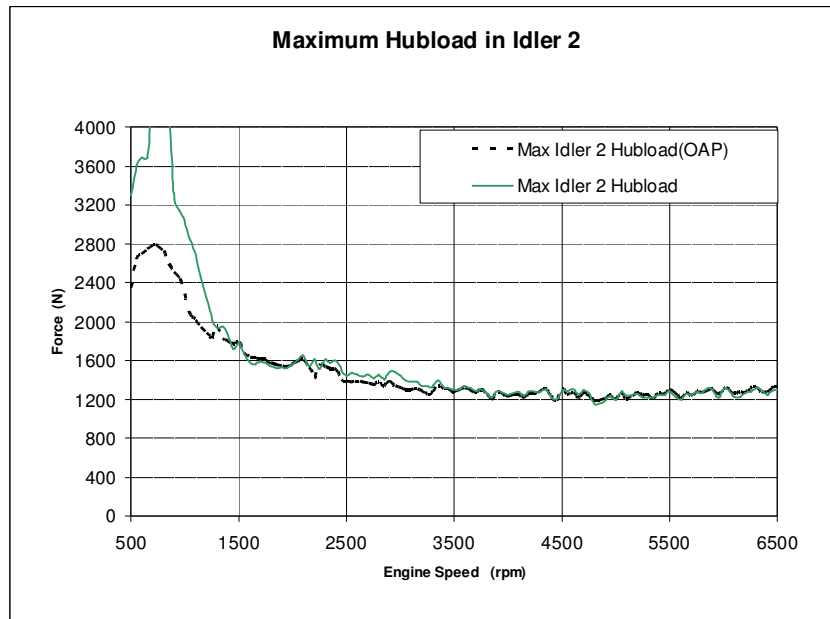
Figure 7. Maximum hubload in idler 2 (comparison between result with OAP and without OAP)
