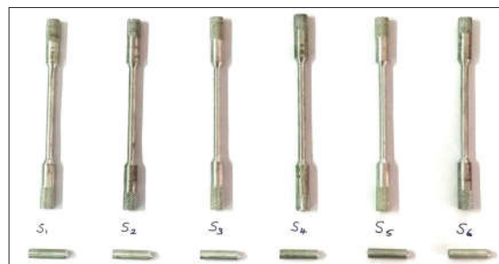
Fig. 3. Tensile and wear test samples
