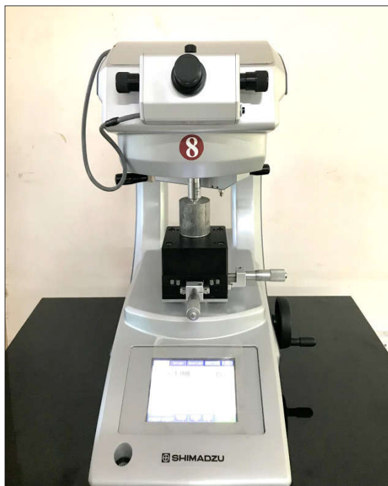
Fig. 2. Specimen loaded on (Shimadzu) hardness tester
