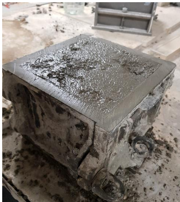
Figure 11. A 150 millimeter mold filled with concrete
