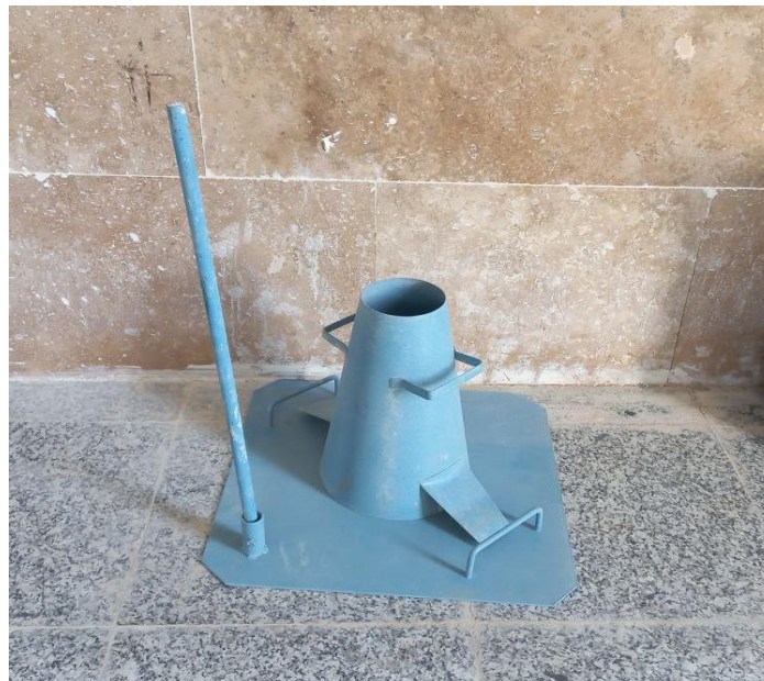
Figure 10. Slump test cone
