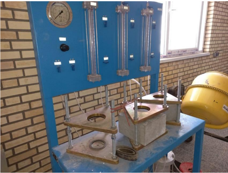
Figure 17 An image of the permeability test apparatus
